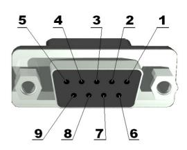
**TXDO** Output **Transmit Data.** This is the asynchronous serial data output (RS232) for the shift register on the UART controller.
