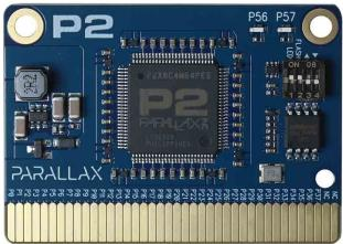
The P2 Edge Module is a simple way to get started with the Propeller 2 multicore microcontroller. In addition to speeding development, this module provides an optimal P2 building block for system integrators and designers to include in their products.
