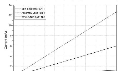
Typical Current of a Cog vs. Operating Frequency (Vdd = 3.3 V, Ta = 25° C)
