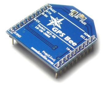
This is a 50 channel GPS module with high performance u-blox 5 engine, all capsule in a mimic popular XBee compatible 20 pin socket.
