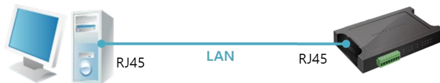
Figure 2-1 the connection between CIE-H14A and a PC
